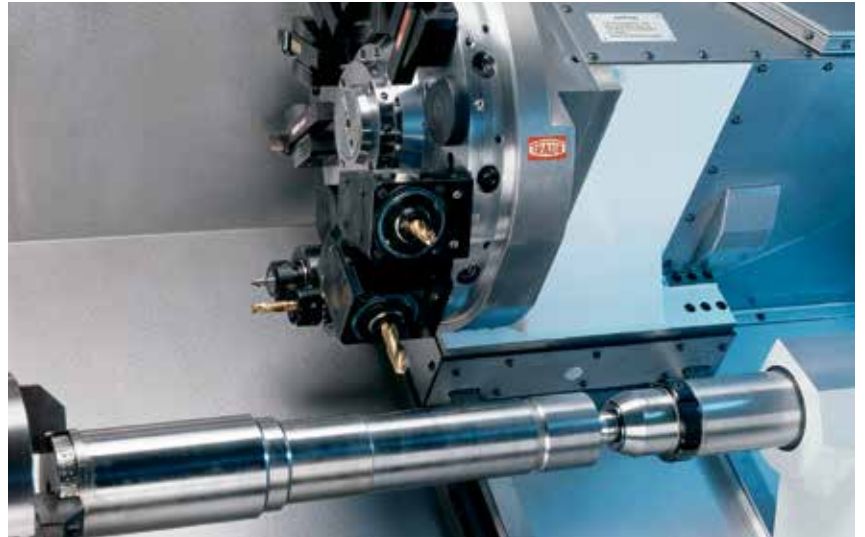
A generously dimensioned tooling zone and a rapid-index disk-type turret with 12 tool reception bores. Internal coolant supply and directional logic are standard.
