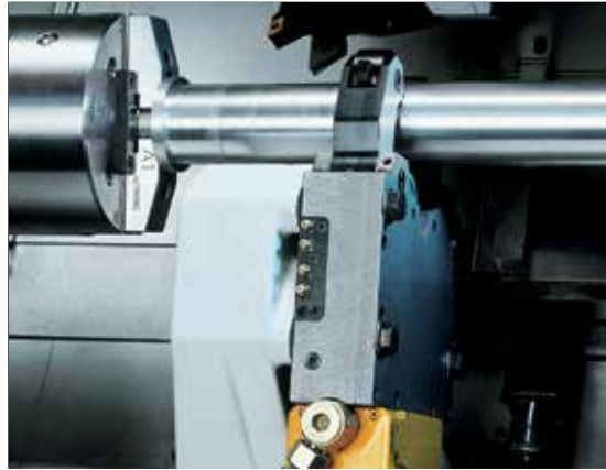
Whether shaft-type, semi-finished or bar components – universal machining is a decisive factor. Photo: fixed steady
