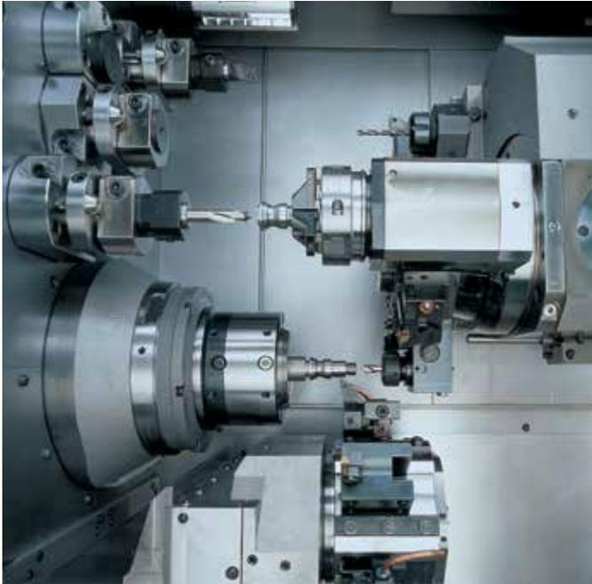
The INDEX ABC has 2 tool turrets with 14 tool mountings. An upper turret with 7 tool stations plus a fixed station for mounting a synchronous spindle (for chuck or collet clamping) and a lower turret with additional 6 tool mountings. Plus five back-boring stations (of which 2 are live) for cutoff-end machining.
