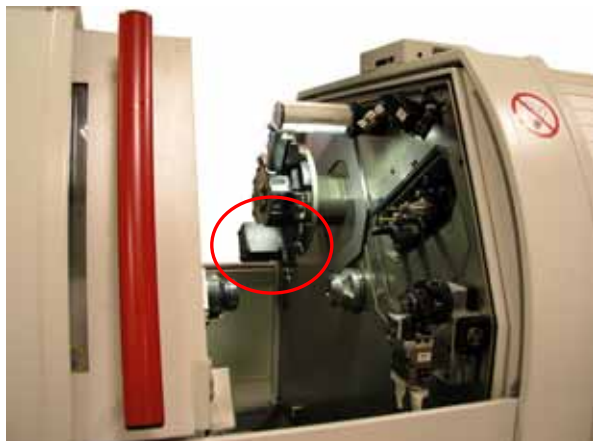
Pic 1: High-frequency tool holder on the upper turret
