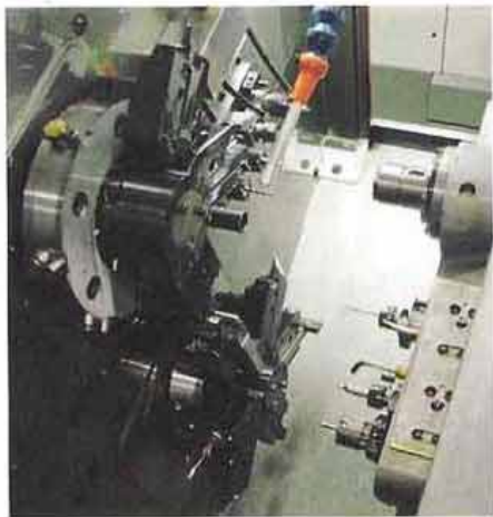
Structure Medical relies on a combination of fixed and sliding headstock turning machines and milling centers for machining complex medical parts.
