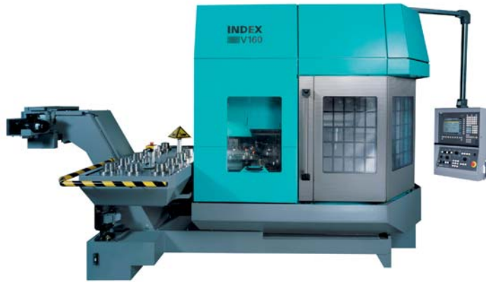
Fig. 1: INDEX V160C: Hard turning and grinding on a single machine
