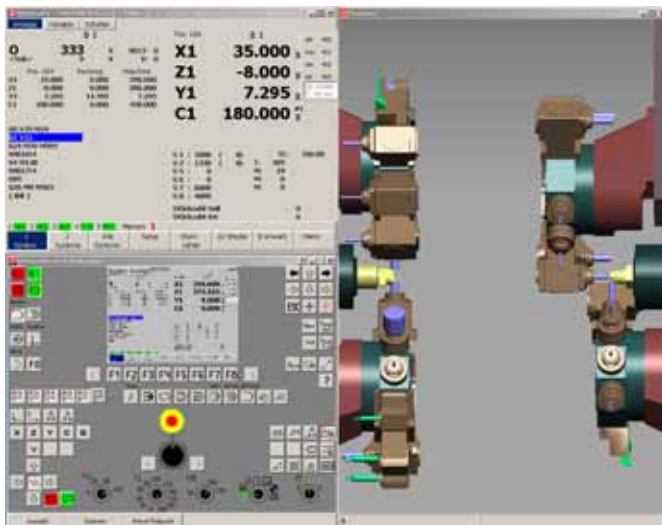
Fig. 1 Screen view WinFlexIPS Plus : Operating panel; machine screen and simulation depicted in a transparent way.
