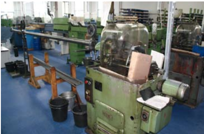
Mechanics – pure and indestructible: Eight A25 type lathes stoically perform their duty at Jowos in Seitingen; the continuous-running machines perform the classic bread-and-butter business with simple bulk parts
