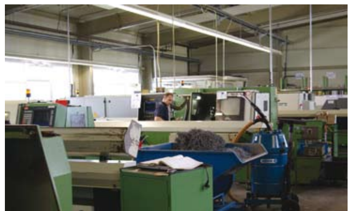
In the modern production hall of Otto Schmid Metallbearbeitung, individual parts and series in large quantities are produced on 11 TRAUB CNC turning machines
