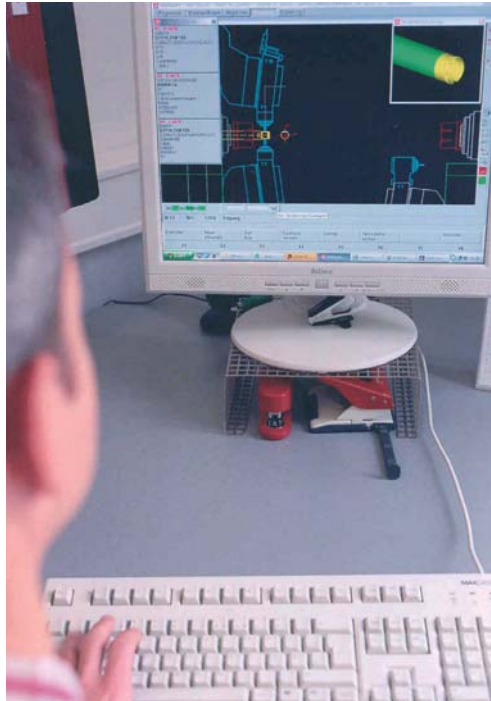
At Kieselmann GmbH, the 'TNX80/65' is programmed run-capable via WinFlex ITS software and checked for collision in the work planning - however, the powerful program for the fine optimization is also available on the CNC panel.
