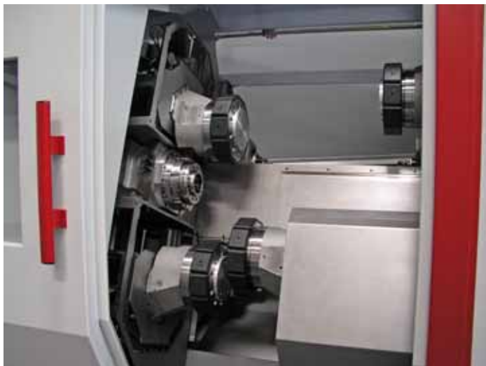
Figure 1: Working area of the TNX65/42 with four turrets: The space for tool change is 250 mm in Z direction and 72 mm in X direction
