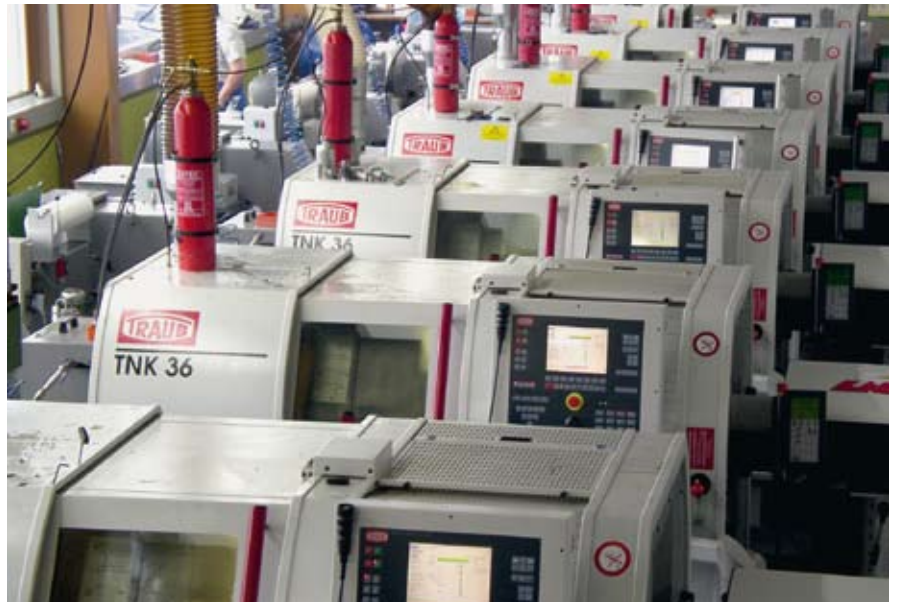
Fig. 1: A powerful squad: The ten TRAUB single spindle bar automatics of the »TNK36« type in rank and file – their compact arrangement ensures short paths in multi-machine operation, access to the working area on both sides, making for short setup times
