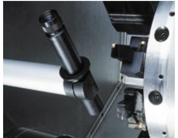
The automatic tool position setting ATC forms an integral part of the basic equipment.
