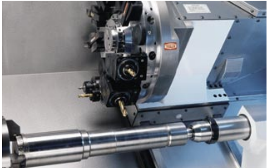
A generously dimensioned tooling zone and a rapid-index disk-type turret with 12 tool reception bores. Internal coolant supply and directional logic are standard.
