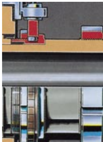
A generously dimensioned tooling zone and a rapid-index disk-type turret with 12 tool reception bores. Internal coolant supply and directional logic are standard.
