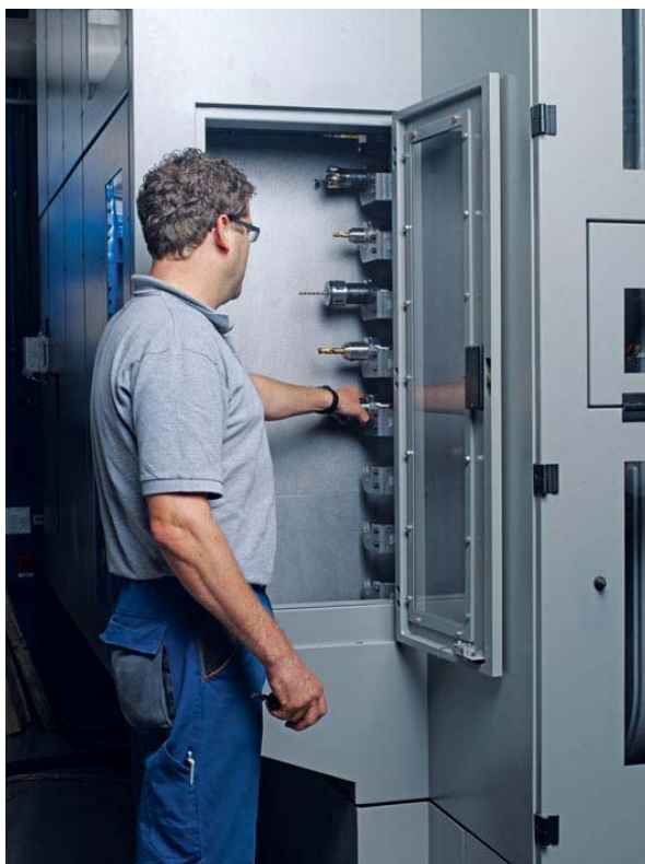
Figure 5: A separate loading strip allows setting up the machine during main time.
