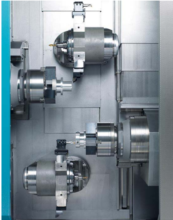
Figure 4: Precise turning operations with stationary tools in the tool strips on the motorized milling spindles
