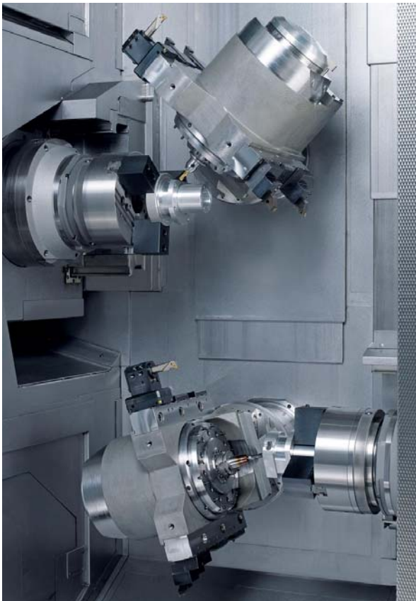
Figure 2: Two work spindles and two motorized milling spindles perform high-productivity machining operations in two independent sub-systems
