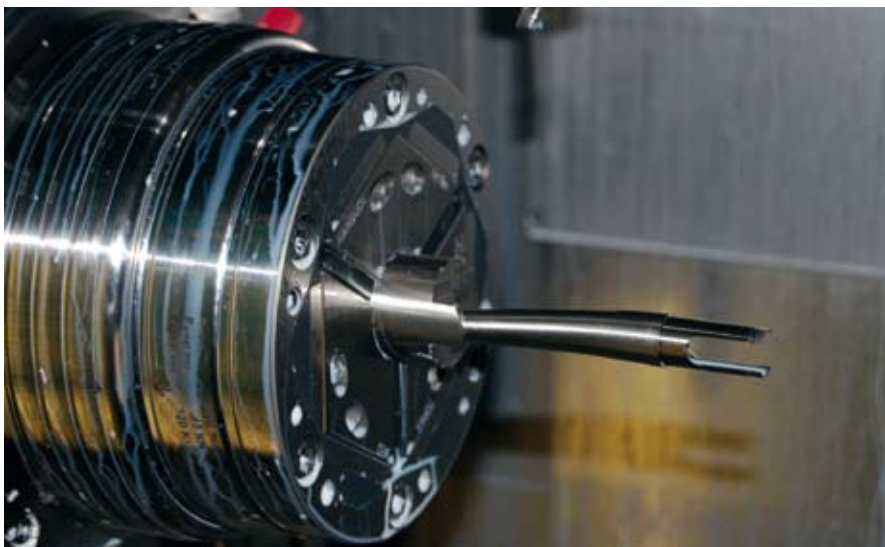
A sophisticated part: The ready-made handle sleeve of the dental instrument is machined at Sycotec.
