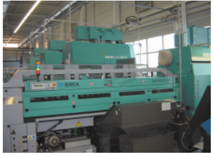
Obligatory: All multi-spindle automatics are supplied via the latest bar loading magazines.
