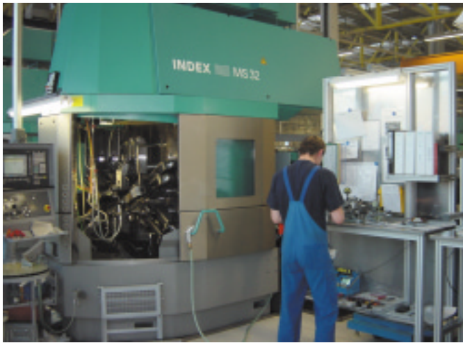
„The MS32 Compact is worldwide the first multi-spindle turning machine open at the front...“
