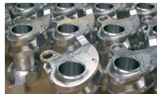
Below: Torsion carrier - highly complex functional parts for the wing division of the Airbus family
