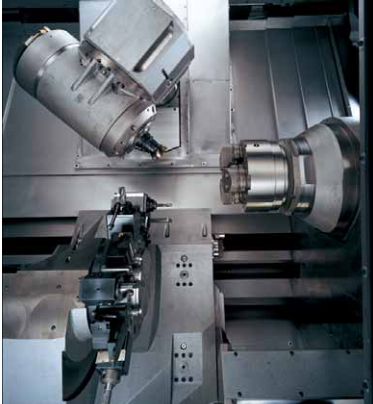
Pic 2: Heavy-duty milling spindle
