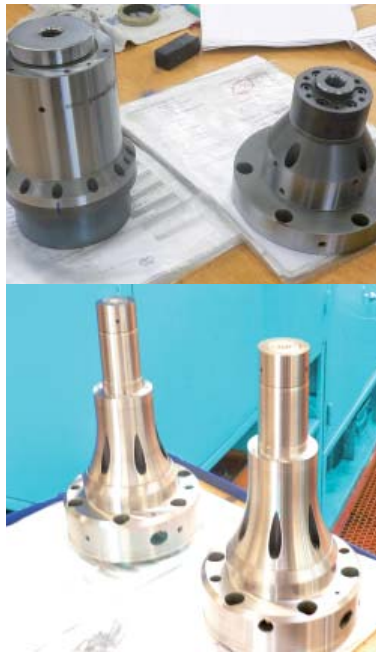
Some examples of clamping mandrels that are completely machined on the INDEX G200 CNC turning centres
