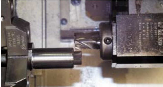
Complex turning with drill mill operations can be combined
