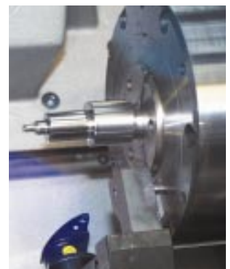
The keyway on the face of the chuck which is used to hold the inner body of the eccentric chuck.
