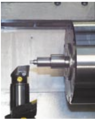
Complex turning with drill mill operations can be combined
