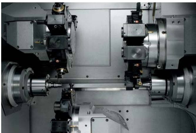
The large tool stock in the three turrets and the standard W-serration of the C100 ensure short setup times even with small lot sizes.
