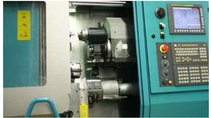
The INDEX ABC automatic production lathe is suitable for complete machining of complex parts. Its ability to engage up to 3 tools simultaneously ensures high productivity levels
