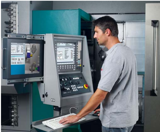
Figure 4: The VPC Box located directly next to the control brings the Virtual Machine or other Windows applications directly to the operator
