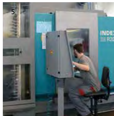
5 Productivity guarantor: efficient complete machining of safety-relevant connectors on the INDEX R200 turn-mill center. © Hanser
