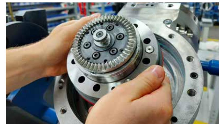
Reliable polygon connections are also used for spindle drives on INDEX and TRAUB machines. The picture shows the 3-sided polygon on the turret drive of the INDEX G220.
