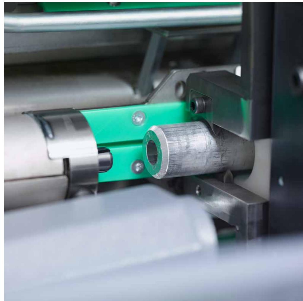
The bar stock is drilled in the bar loading magazine during machining. This enables continuous, fully enclosed guiding of the bar stock.
